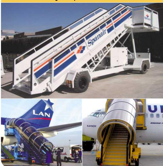
The Self-propelled Universal Passenger Step, model EDU, has been designed for embarking and disembarking passengers on all and W.B. conventional aircraft with sill heights ranging from 2.45m to 5.80m (front door of B737 to rear door of A-340)
